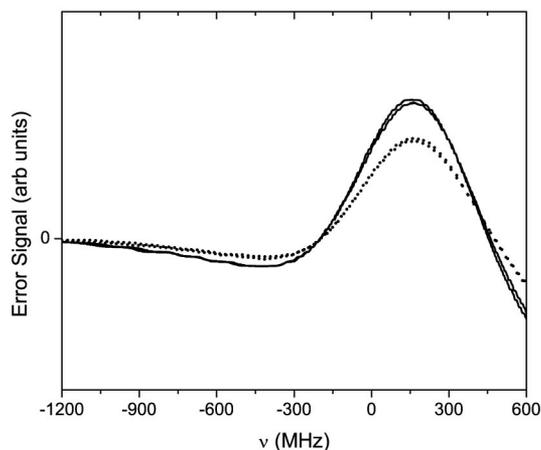
Fig. 2. Temperature sensitivity of DAVLL error signal. The solid traces were measured at a temperature of 26 °C and the dashed traces at 20 °C, for the same polarization settings as in Fig. 1. Two traces are shown at each temperature.
