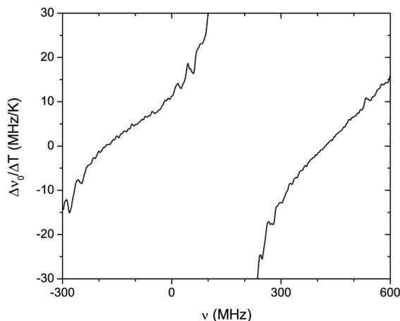
Fig. 3. Temperature sensitivity of DAVLL lock. Using scans such as Fig. 2, the sensitivity of the laser lock frequency  $\nu_0$  to temperature  $T$  is derived, as described in the text. The temperature sensitivity diverges at the extrema of the error signal curve, here at approximately -400 MHz and +150 MHz. It is not possible anyway to lock the laser near these points because the error signal slope is too small.
