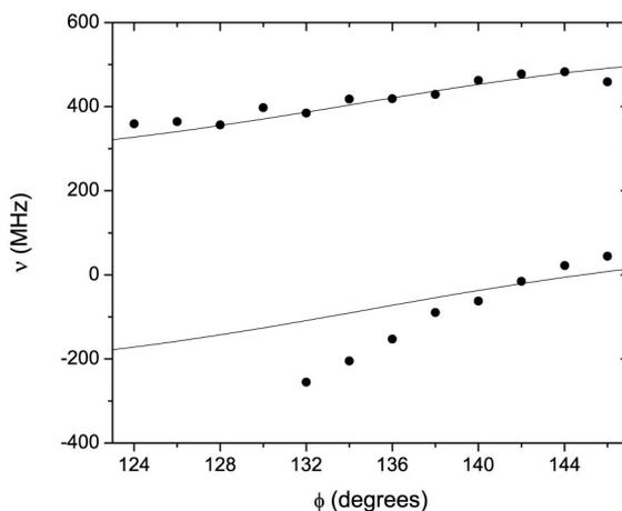
Fig. 4. Location of TIPs. The data points indicate frequencies where the DAVLL is measured to have zero temperature sensitivity, plotted as a function of wave-plate angle  $\phi$ . The input polarizer angle  $\theta$  was held at  $90^\circ$  and the optical attenuation was adjusted to give zero error signal off resonance. The solid curves show the location of TIPs predicted by the model.
