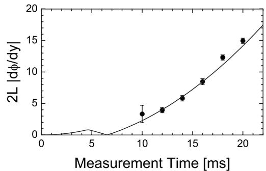
FIG. 3. Magnitude of the phase gradient for a single-sided interferometer of total duration  $2\tau_1$ . Points show the experimental measurements, with error bars determined by the fitting procedure. The curve shows the results of the calculation described in the text, with the gradient scaled to the length of the packet,  $2L$ .
