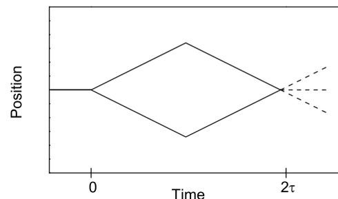
FIG. 1. Packet trajectories for the single-sided interferometer configuration. At time  $t=0$ , a Bose-Einstein condensate is split into two wave packets that move apart with velocities  $\pm v_0$ . At time  $\tau$  the packets are reflected, and at time  $2\tau$  they are recombined. The resulting state depends on the phase difference between the paths. In actuality, the trajectories will be distorted by the weak harmonic potential in which the packets move.
