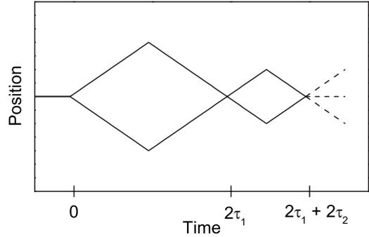
FIG. 5. Packet trajectories for the double-sided interferometer configuration. The packets are split at time  $t=0$ , reflected at time  $\tau_1$ , reflected again at time  $2\tau_1 + \tau_2$ , and finally recombined at time  $2\tau_1 + 2\tau_2$ . For a symmetric interferometer with  $\tau_1 = \tau_2$ , the phase gradients on the packets are nearly eliminated.
