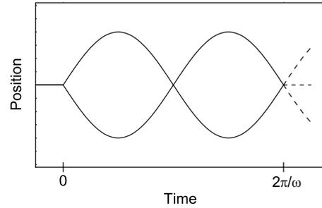
FIG. 8. Packet trajectories for the free-oscillation interferometer. The packets are split at time  $t=0$  and then complete a full oscillation in the harmonic guide potential before being recombined. Here  $\omega$  is the oscillation frequency in the guide.
