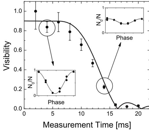
FIG. 4. Visibility of the single-sided interferometer, as a function of total duration. Points show the measured values, while the curves show the theoretical estimation using the rigid packet model. The prediction has been scaled by 0.9 to account for experimental imperfections that are expected to be independent of duration. The insets show example interference curves at the points indicated.
