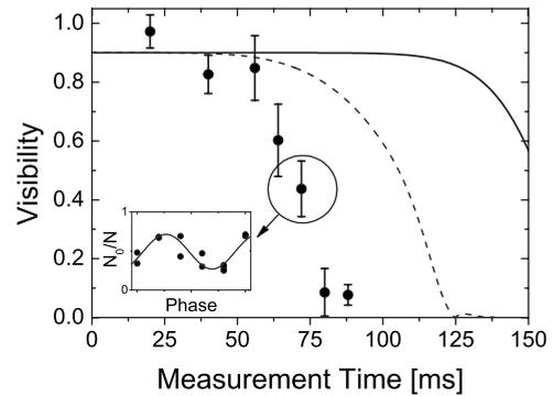
FIG. 7. Visibility of the symmetric double-sided interferometer, as a function of the total measurement time  $T = 4\tau$ . Data points show the experimental results and the curves show the predictions of the rigid-packet model (solid) and a dynamic packet model (dashed) [15], each scaled by 0.9 as in Fig. 4. The inset shows an example interference curve at  $T = 72$  ms.
