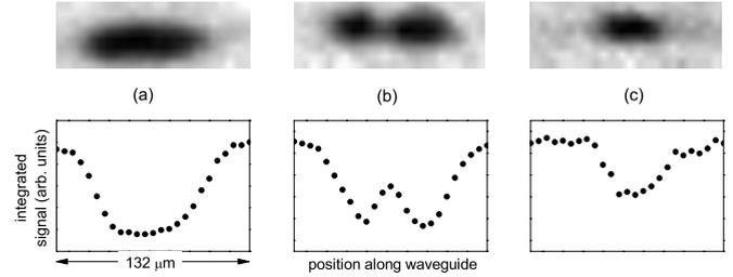
FIG. 2. Absorption images of wave packets used in the condensate interferometer. (a) The condensate distribution, before the interferometer operation. (b), (c) Packets observed in the interferometer output, for two different phase offsets  $\theta$ . The graphs show the absorption signals integrated along the transverse direction, which are analyzed to determine the modulation period and thereby the phase gradient.
