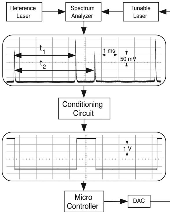
FIG. 1. Schematic of a lock system. Beams from a stabilized reference laser and a tunable laser are sent into a spectrum analyzer. The upper graph shows a typical output signal. The conditioning circuit of Fig. 2 converts this to a digital signal as shown. The microcontroller inputs the signal, calculates the feedback voltage, and applies it to the tunable laser via a digital-to-analog converter.
