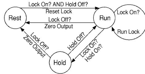
FIG. 3. State diagram of the control program. Circles represent states and arrows represent transitions. Transitions are labeled with their conditions and commands.
